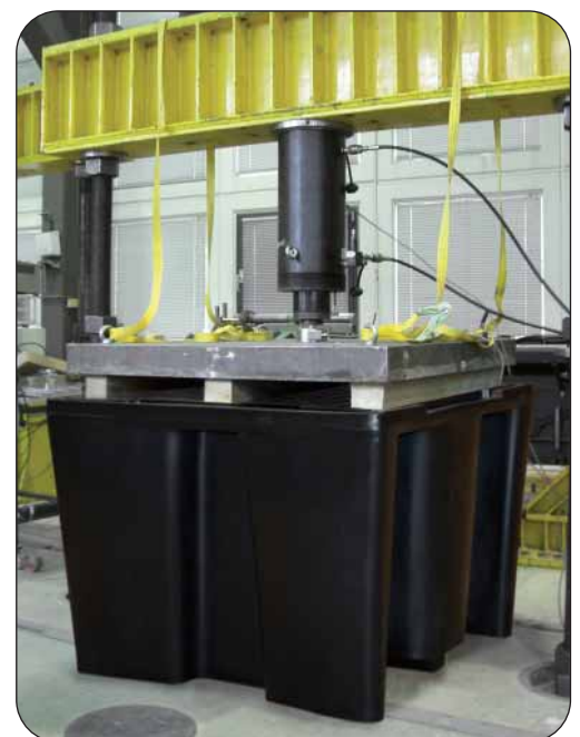
PE-KT-1 under a test load of 8.000 kg
