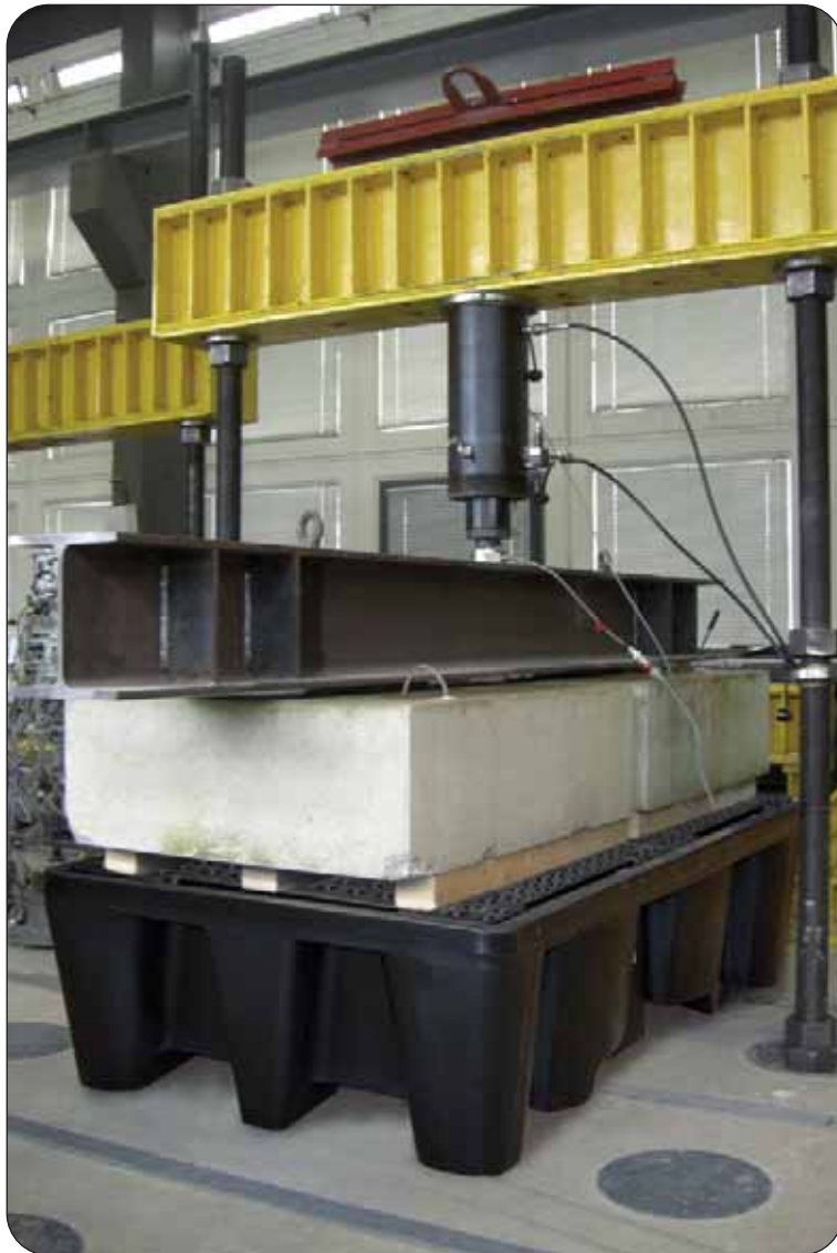
PE-KT-2 under a test load of 16.000 kg
